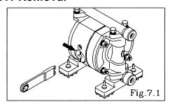
Remove the cap using the cap and disk remover. (special tool: Part No. 771132). [Fig.7.1]
