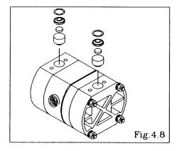
Remove the O ring, valve seat, flat valve and valve stopper.[Fig.4.8]
